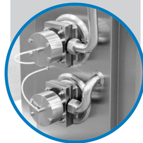
Dettaglio pompe a lobi/ lobe pump detail
